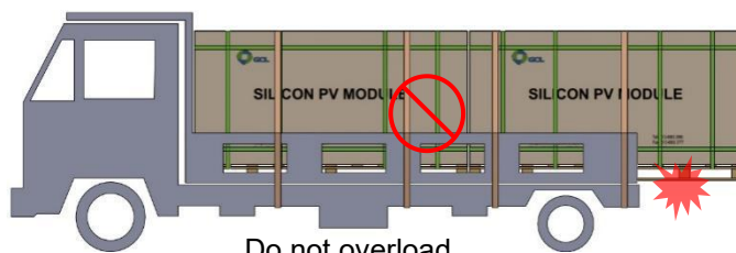
Do not overload
